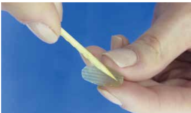
FIGURE 1: Application of a thin layer of cyanoacrylate glue on the plastic sheet with the aid of wooden toothpick
