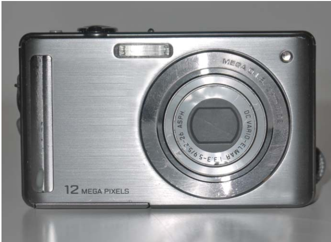
FIGURE 12: Compact Camera—dimensions: (length x depth x height): 9 x 2 x 5.5 cm. Property of the author
