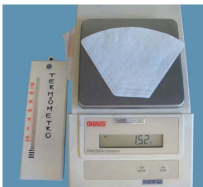
FIGURE 2: Thermometer and precision scale used in the gravimetry test
