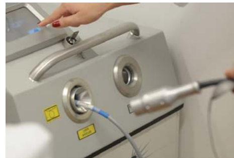
Figure 2 - The Xtrac® hand piece is flexible, articulated, and has an area of 4cm 2
